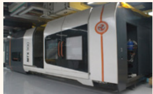
Precise 5 axis Multi-Tasking Machine (2 ATCs with capacity of 120 different tools)
